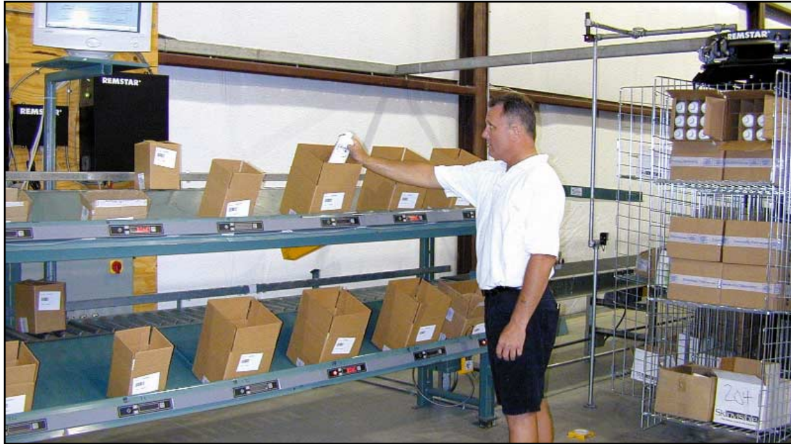
Automated universal workstation consisting of horizontal carousels and pick-to-light flow rack provides four to six hour order processing at up to 700 lines per hour.
